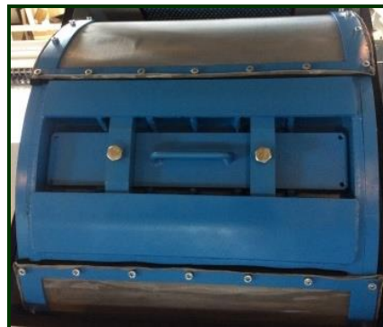
Residues unloading nozzle
